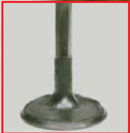
Intake valve after P.i. treatment
